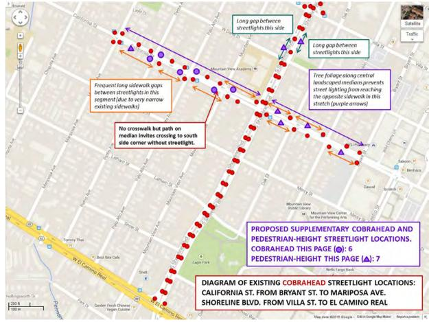
FIGURE 48: STREETLIGHT LOCATIONS ON SOUTH SHORELINE AND CALIFORNIA STREET (EASTERN PORTION)
