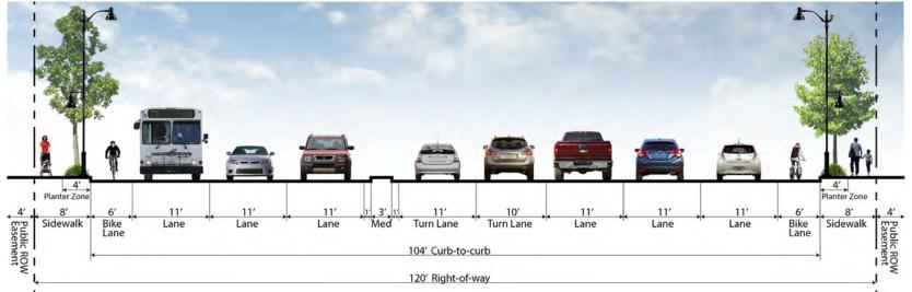
Figure 3-2: Typical Street Cross Section - Class II Bike Lane
