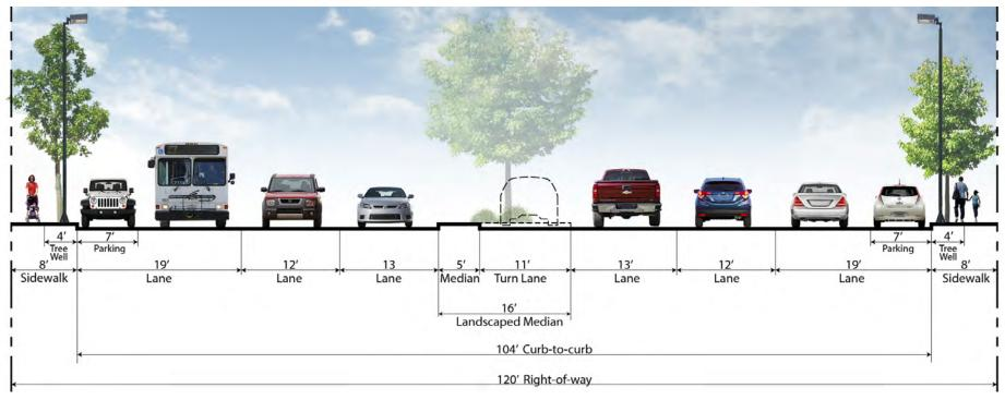
Figure 2-1: Existing Conditions Street Cross Section
