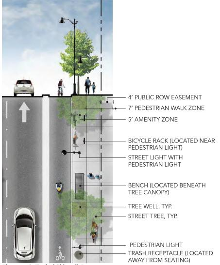
*Figure 3-18: Typical Sidewalk Layout All improvements shown are conceptual and subject to further study and refinement.*
